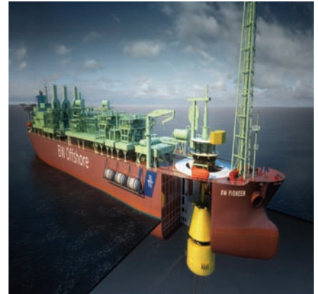
For ultra-deep water (> 7,500 ft), the future will likely see the continued use of the robust semisubmersible solutions (left) and, increasingly, the use of floating production, storage and offloading vessels (FPSOs) such as that adopted for the Cascade/Chinook development (right).
