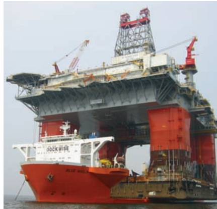
For ultra-deep water (> 7,500 ft), the future will likely see the continued use of the robust semisubmersible solutions (left) and, increasingly, the use of floating production, storage and offloading vessels (FPSOs) such as that adopted for the Cascade/Chinook development (right).
