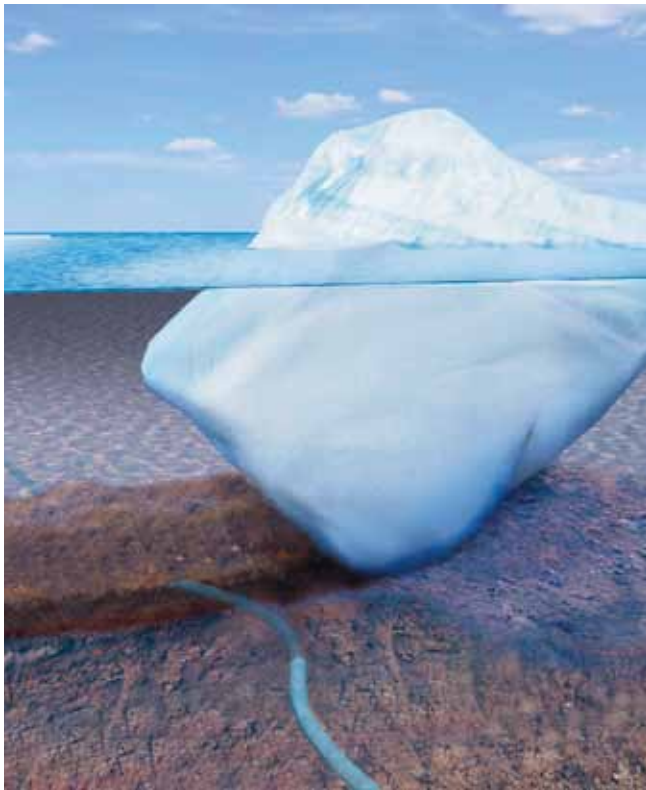
Figure 1. Artistic illustration of pipeline gouging showing deformed pipeline beneath ice gouge.
