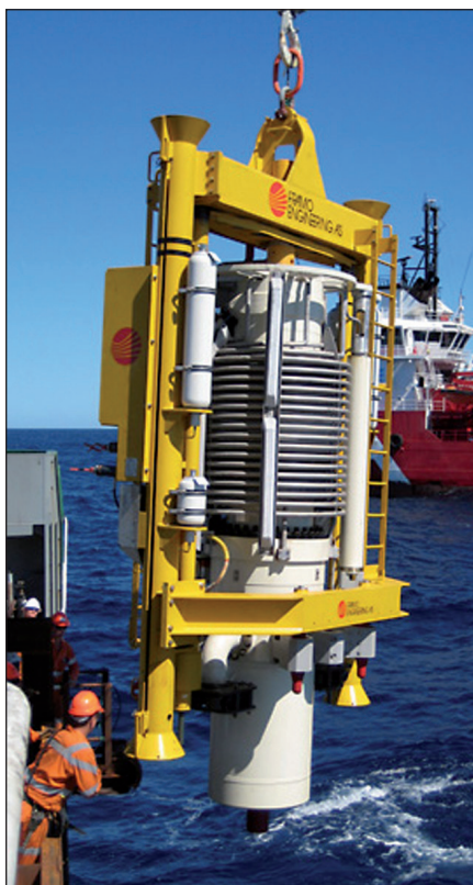
Frontier developments in cold climates require robust subsea systems, such as hybrid pumps. The Framo hybrid boosting pump pictured adds pressure to a subsea system to improve production efficiency from a subsea well to a host facility.
