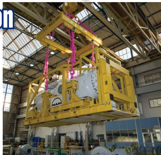
The subsea gas compressor for Statoil's Åsgard field, which is scheduled to start production in 1Q 2015. For more details on current subsea processing trends and technologies, see the poster included in this issue. (Image courtesy MAN Diesel & Turbo)
